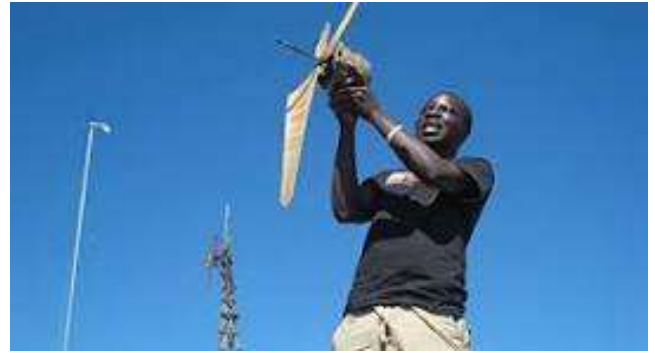
William uses an old iPod Nano motor to test his idea
